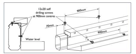
Minimum frame requirement Louvre box gutter
